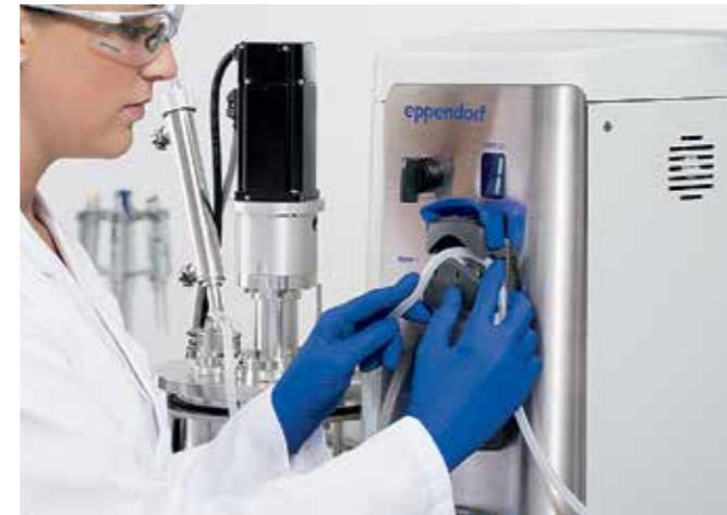
Variable/fixed speed front-mounted pumps are capable of clockwise and counterclockwise rotation.
