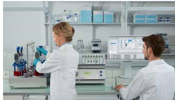
The parallel design of DASware control allows for the operation of a DASGIP Parallel Bioreactor System with up to 16 vessels.
