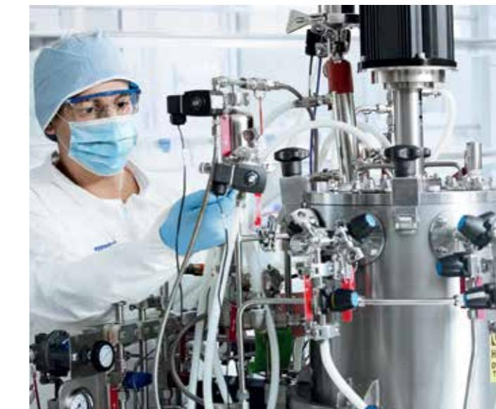
Numerous ports in the vessel head plate and sidewall provide flexibility to position sensors, spray balls, addition valves, pressure transducers, and more.
