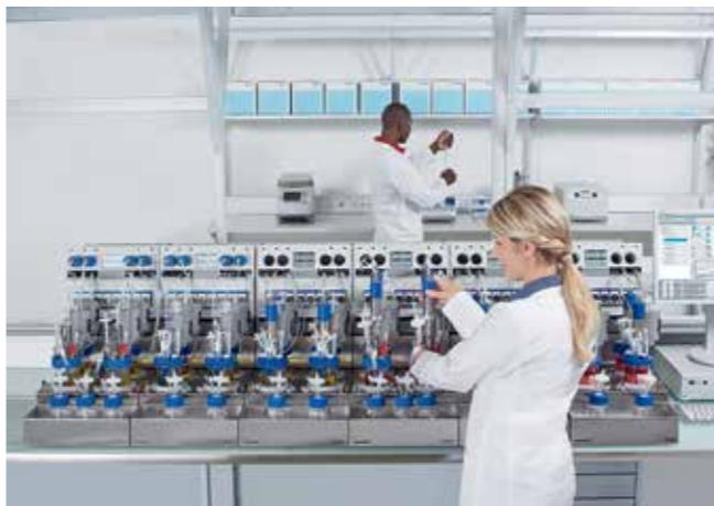
Parallel operation of up to 24 bioreactors makes the DASbox a perfect fit for process development.
