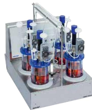
The compact DASGIP Bioblock provides independent temperature control and can be operated with BioBLU 1 Single-Use Vessels.
