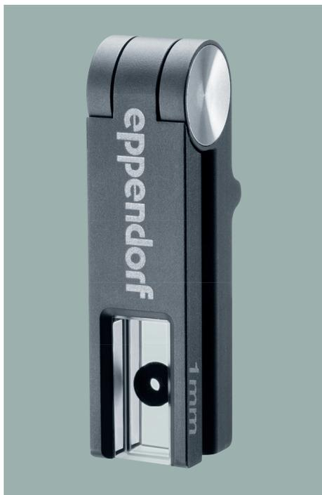
With an optical path length of only 1 mm, the  $\mu$ Cuvette G1.0 features a light path that is ten times shorter than the light path on standard cuvettes. This allows high nucleic acid and protein concentrations to be measured using the  $\mu$ Cuvette G1.0. Only 1.5  $\mu$ L of a sample is required for the measurement. The  $\mu$ Cuvette G1.0 offers a flexible expansion of the photometric application range of Eppendorf photometers.
