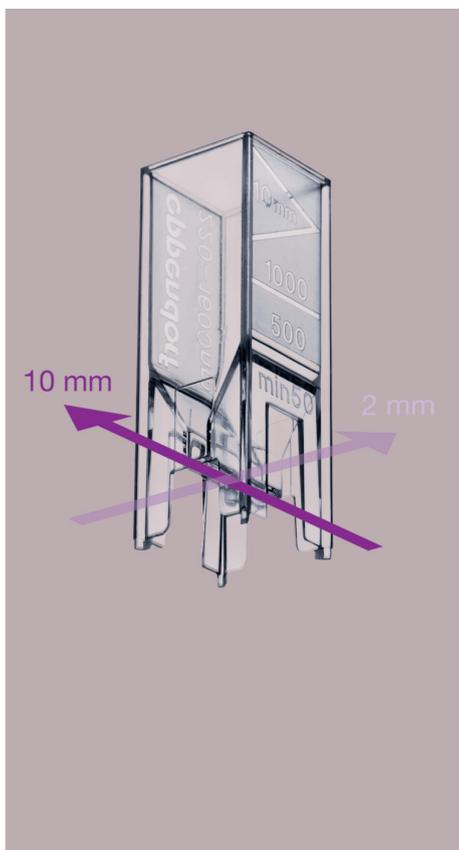
The patented\* Eppendorf UVette is a fully UV-transparent, single use cuvette made of clear plastic, with a light transmission of 220 nm to 1,600 nm. The unique design allows you to conduct flexible measurements with two different light paths (10 mm and 2 mm).
