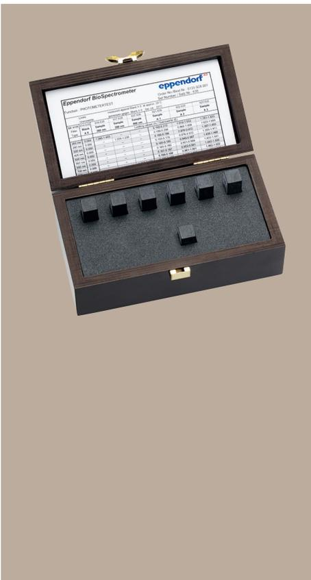
The secondary UV/Vis reference filter set is used to verify the photometric and wavelength systematic errors according to NIST® (National Institute of Standards and Technology, Gaithersburg MD, USA).
